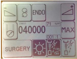
Screen of brushless micromotor taken with fiber optic switched on and water spray to the instruments controlled from the pedal active:
