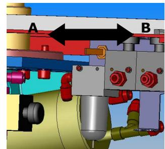
Pressure reducer that pressurizes the little tank that distributes the water to the handpieces during the replenishment of the mixer tank regulated at 2 bar pressure
