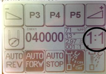
DISPLAY WITH FUNCTION "TORQUE" ON - TORQUE CONTROL ( IN N/CM)
