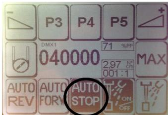
**MICROMOTOR function with "AUTO STOP" program on :** when you move the pedal lever to the right, the micromotor rotates clockwise, it stops when it reaches the torque set.
