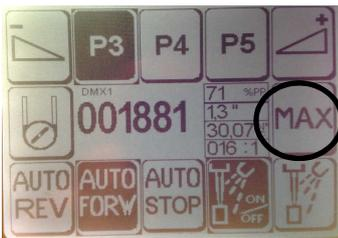
DISPLAY WITH FUNCTION "1:1" ON - TRANSMISSION RATIO CONTROL OF THE INSTRUMENT IN USE
