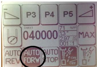
**MICROMOTOR function with "AUTO FORW" program on :** when you move the pedal lever to the right, the micromotor rotates clockwise, it stops when it reaches the torque set, starts the rotation in reverse for the TIME set and returns to turn in a clockwise direction. The cutter reverse starts every time when it reaches the torque set .
