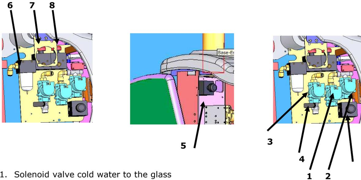
1. Solenoid valve cold water to the glass
